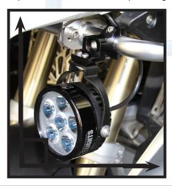
Passengers and luggage may alter the alignment of the light, so further adjustments may be needed. You may find that a slight downward angle (5 degrees at most) is helpful. Often times it is helpful to angle the right side light toward the right side of the road. This helps with identifying road terrain and potential critters.
