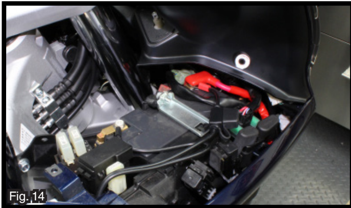
Run the red and black power wires directly to the battery. Make sure fuse is disconnected before attaching wires. (Fig. 14)
