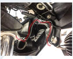
10. Align and level the lights, on flat ground, with a rider on the bike. Reassemble the tank body work, and side panel fasteners. Connect the battery wires to the terminals, fit the seat back onto the bike. Ensure the bike starts and that the lights operate as expected. Congratulations! You have completed the installation of your Clearwater Lights!
