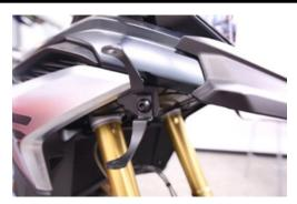
9. Fasten your Clearwater Lights to the mod bracket, connect the light wires to the harness. Use zip ties to neatly route the wires away from all moving parts and possible pinch points around the front end. Make sure the wires coming out of hte Clearwater Light are not being pulled, but are relaxed. Red line showing path of light wires under beak.
