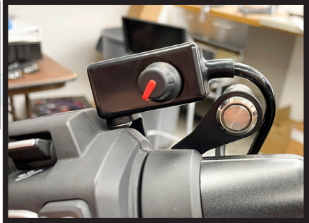
Dimmer and switch mounting location
