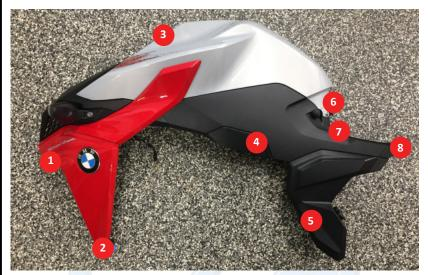
Tips: Fastener 4 denoted in the photo above utilizes a T30 Torx, otherwise all other OEM fasteners use a T25 Torx wrench. Fasteners 7 & 8 are slightly longer than all of the others. Fastener 1 is accessible from the inside.
