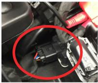
Plug the data cable into the mating connector on the CANopener (green connector) and ensure it is plugged into the harness at the front of the bike as well. Neatly bundle any excess wires with a couple zip ties and mount the CANopener in the area in front of the battery with the attached velcro. Remove the the fuse from the fuse holder and attach it to the red wire from the harness. The power wires can be connected to the battery.
