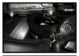
• Zip-Tie the cables from the lights as shown to the brake unit mounting bracket as shown. Verifying that there is enough slack in the cables to not interfere with turning or the shock movement.
