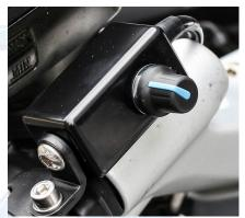
**Hint for High Vibration installations:** To keep the Volume Control Knob from rotating itself under high vibration, put a dab of silicone adhesive under the knob and let it dry. Then push the rubber knob back on. The friction of the glue under the knob will keep it in place.
