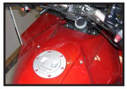
• Gas tank battery cover removed. (*Disregard Touratech Canbus helper shown, not part of installation*).
