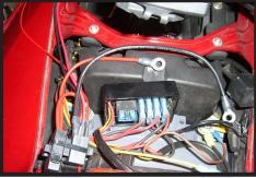
• Remove the fuse, connect the harness to the battery, black to negative (-) and red to positive (+).
