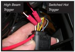
• Install supplied Posi-Taps on to the YELLOW/WHITE wire which is used for the SWITCHED HOT trigger for the Clearwater Lights harness (RED). For the high beam feature, connect the WHITE wire from the volume control knob to the WHITE wire on the connector.
