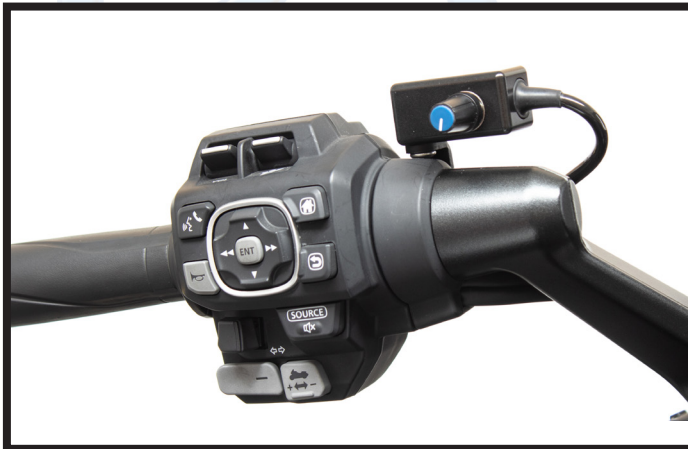
Dimmer mounting location on left side of handlebars
