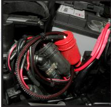
Wire routing suggestion: Tuck away excess CANbus harness wire in the right fairing as shown.
