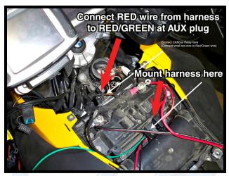
Horn Feature: Locate the high beam wire on the bike. Posi-Tap the WHITE wire from the harness to the WHITE wire of the high beam circuit wire. This will make the Clearwater Lights go to 100% when the high beam is on.
