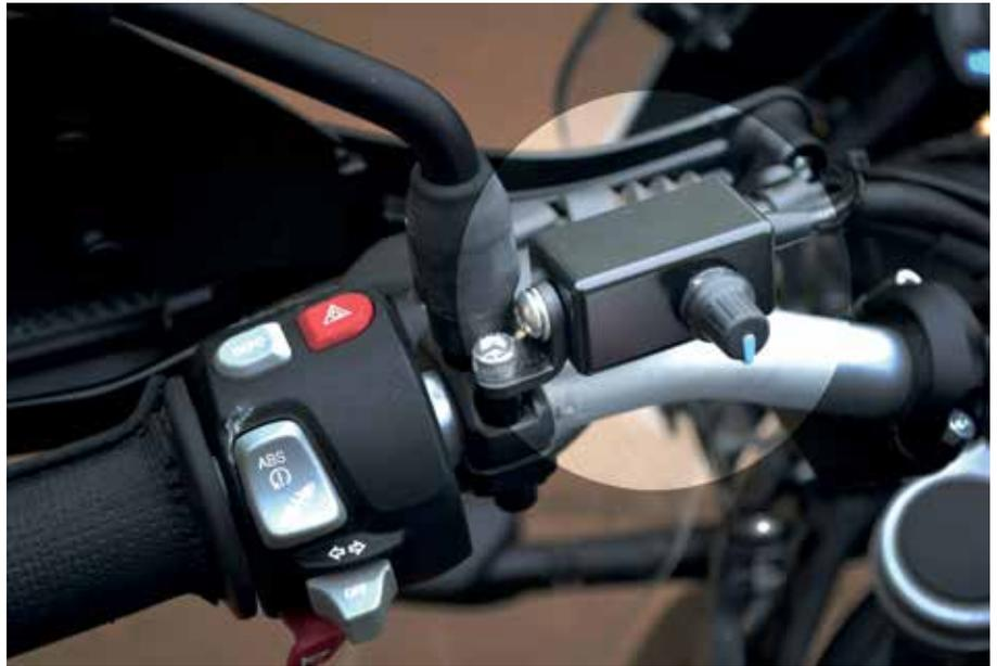
The Darla Universal Kit from Clearwater Lights includes a unique, handlebar-mounted dimmer to regulate the lights' brightness from 5 to 55 percent. The auxiliary lights can be boosted to full, 2,000 lumens power by toggling the bright beam switch.
