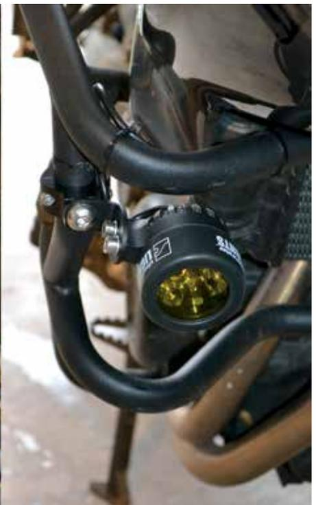
Clearwater Lights can provide custom mounts for front forks or engine guards.
