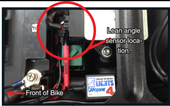
CANopener location on a K1600GT.
