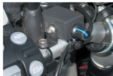
Top: Mounting hardware with Kristas. Bottom Left: Kristas illuminated on Ray's GS. Bottom Right: Dimmer knob as mounted on left handlebar, near mirror mount.
