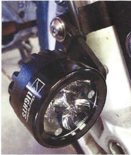
Fork leg brackets were used to mount the two-inch, 2,000 lumen Darla lights.
