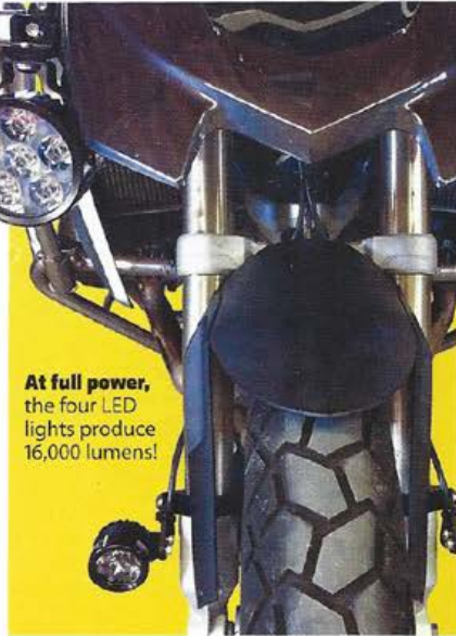
Fork leg brackets were used to mount the two-inch, 2,000 lumen Darla lights.
