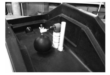
**Step 14**Put the drain plugs in from the inside and install the float assembly with the <sup>1</sup>/4" thumb screw. Fill the tank up to the top of the gasket on top of the base. The valve should shut off. When setting, use pliers to tighten the thumb screw. Then secure the top to the base and you're finished.
