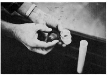
**Step 6** Remove the rubber washer from the  $^{3}/_{4}$ " female adapter and set aside for use later.
