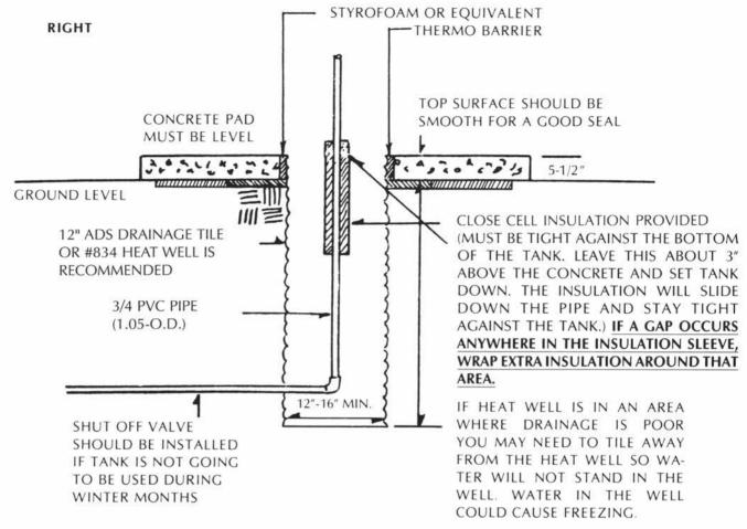
IF USING BLACK ABS PLASTIC PIPE, USE A PLASTIC NIPPLE WITH 3/4" THREADS TO MAKE THE TRANSITION TO THE 3/4" PVC PIPE PROVIDED. METAL FITTINGS ARE NOT RECOMMENDED.
