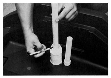
**Step 4**Make a mark on the  $^{3}/_{4}$ " PVC pipe even with the top of the  $1^{1}/_{2}$ " pipe. Then remove the top  $1^{1}/_{2}$ " fitting. Merely pull it out, it is not glued. Measure down  $^{1}/_{4}$ " from your original
