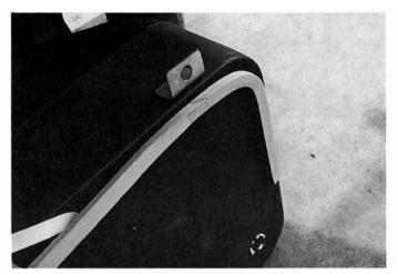
**Step 2** Clean base and install your adhesive backed gasket material to the bottom of your base assembly.
