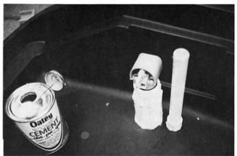
**Step 13**Screw the valve in tight into PVC fitting. Hand tight is usually enough.
