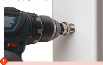
**WARNING:** Do not use an impact driver or you risk damaging the set screw channel and increasing the likelihood of seizing during installation.
