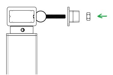
12 Insert the pivoting screw into hinge part C so that part B fits into the curved bed. Secure loosely with the nut.
