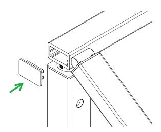
22 Slide in the end cap at your corner hinge making sure the notch accommodates the screw holding the hinge to the side of the handrail.
