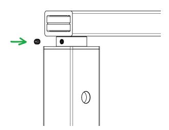
If necessary, use **Fixed Straight Spline** instructions on **page 6** to connect your handrail assembly to the previous handrail length. Secure your post top to the post by driving in the set screw with a 1/8" Allen wrench.
