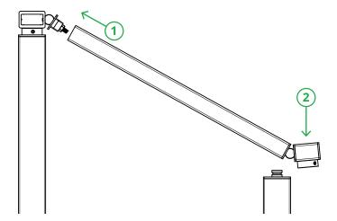
20 Slide this handrail and stair end assembly onto the Handrail Hinge at the other side of the run and lock it in place by fitting the stair end post top collar onto the center pin.
