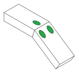
Using a 3/8" drill bit (or appropriate), create three counter sink holes on the spline. These will house the head of the screws. Drill your holes as high as possible to maximize engagement on both sides of the spline.
