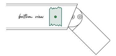
On the underside of the handrail, secure the spline by drilling a 1/2" deep pilot hole using a 5/32" drill bit. Tap the pilot hole using the 10-24 tap. Drive in a 10-24 x 1/2" set screw by hand using a 3/32" Allen wrench.
