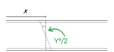
3 Y°/2 will be the angle of your miter cut. Mark this angle on your handrail piece bi-secting the mark you made in **step 1.**
