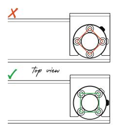
Insert the post top collar into the template and use the set screw cutouts to position the holes in a **square** formation rather than a diamond so you don't interfere with your end cap.
