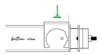
For an end post: Find the location of your post top by aligning the edge of the Handrail Drill Guide and Template flush with the cut of a piece of handrail. Clamp in place.
