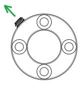
Back the set screw out of the post top collar using a 1/8" Allen wrench until it protrudes slightly. This will prevent the post top from rotating inside the template.
