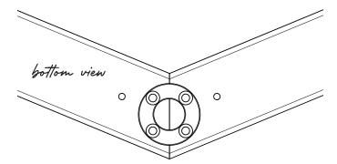
Remove your handrail and place it upside-down on your drilling surface. Attach the post top collar through the corner spline using the **End Post Tops** instructions on **page 25.** Make sure to drill your pilot holes deep enough into the spline to clear the 3/4" screws.
