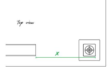
1 Find the length of your handrail by measuring to the far side of your corner post (X). Mark this length on a piece of handrail.
