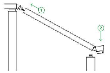
Slide this handrail and stair end assembly onto the Handrail Hinge at the other side of the run and lock it in place by fitting the stair end post top collar onto the center pin.
