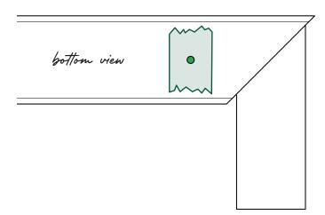
On the underside of the handrail, secure the spline by drilling a 1/2" deep pilot hole using a 5/32" drill bit. Tap the pilot hole using the 10-24 tap. Drive in a 10-24 x 1/2" set screw by hand using a 3/32" Allen wrench.
