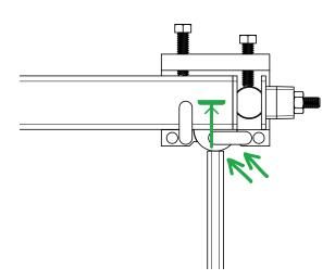
10 For a line post: position the post top so the screws will face away from the stairs, and replace your handrail back on your posts. (If necessary, use **Fixed Straight Spline** instructions on **page 6** to connect your handrail to the previous handrail length.)
