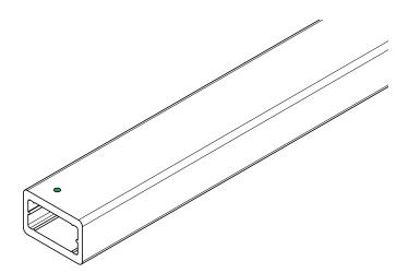
2 Drill a pilot hole using the 11/64" bit. If your post top will be installed into an aluminum spline, drill 1" deep and tap the pilot hole using the 10-24 tap. If it will be installed into a delrin spline or without a spline, drill 1/2" deep.
