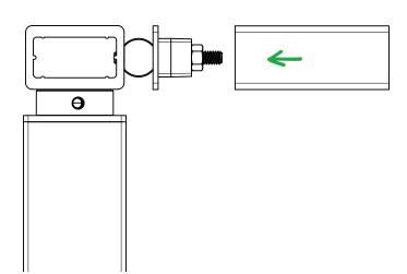
Loosen the nut on one of the Handrail Hinges slightly to allow for adjustment, and take a piece of scrap handrail material and insert it over hinge part C. This will serve as a placeholder when setting the angle.
