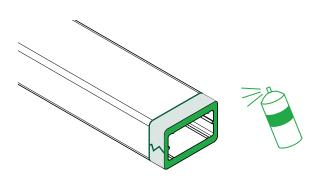
Before removing painter's tape, lightly spray your exposed ends with touch-up paint to cover any blemishes and minimize the appearance of seams. Remove the painter's tape.
