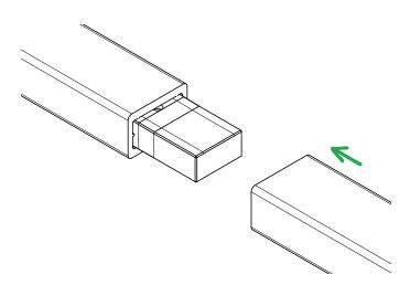
Slide a new length of handrail over the exposed end of the spline and repeat **step 2**.
