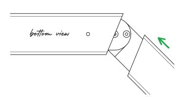
To complete your corner, flip the off-cut piece of handrail from your first miter cut over and fit it to the installed spline. If your off-cut piece is shorter than one foot, cut a fresh length of handrail at a matching angle to complete the transition. Secure by repeating **step 7.**
