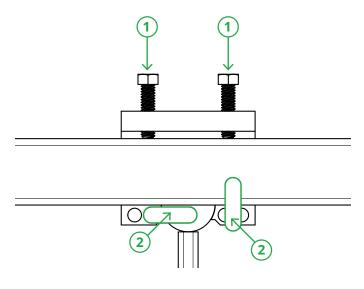
Secure the handrail to the line post top using the Handrail Clamp for Line Posts. Tighten the nylon top screws first and then position and tighten one foot onto the post top and one onto the handrail.
