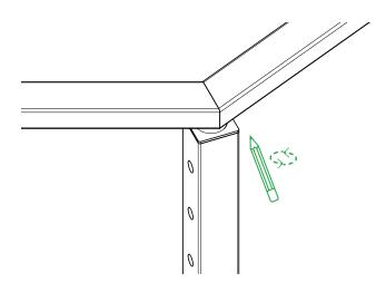
Align the handrail assembly on the post as it will be once installed and mark the location of the post top collar by tracing around it with a fine-point pencil.
