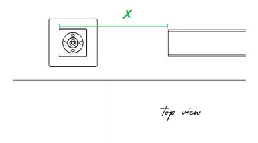
Working from the level section towards the stair transition, find the length of your handrail by measuring to the far side of your corner post (X). Subtract 1/8". Mark this length on a piece of handrail.
