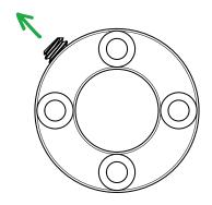
2 Back the set screw out of the post top collar using a 1/8" Allen wrench until it protrudes slightly. This will prevent the post top from rotating inside the template.
