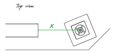
Find the length of your handrail by measuring to the center of the post top on the corner post (X). Mark this length on a piece of handrail.
