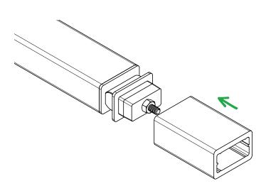
Loosen the nut on one of the Handrail Hinges slightly to allow for adjustment, and take a piece of scrap handrail material and insert it over hinge part C. This will serve as a placeholder when setting the angle.
