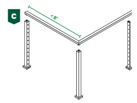
When your entire railing is assembled, secure all end post top collars to center pins and check all line posts for secure handrail connections.
