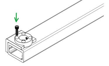
Replace the post top collar into the template and secure it to the handrail using a Signature Series Handrail Mounting Screw and a 5/32" driver.
