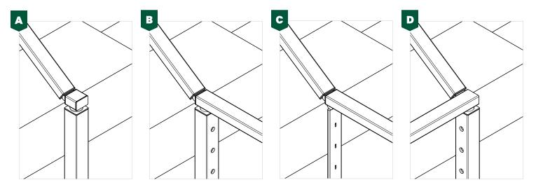
If your stairs end your run, construct a **Stair End with a Handrail Hinge** (**A**) by following the instructions on page 22.
