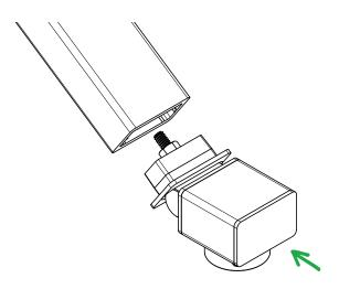
Slide one end of this piece of handrail over hinge part C of the stair end.
