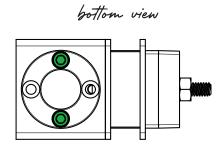
Attach the post top collar to the stair end by driving two handrail mounting screws into the two pre-tapped holes using a 5/32" driver.
