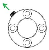
Back the set screw out of the post top collar using a 1/8" Allen wrench until it protrudes slightly. This will prevent the post top from rotating inside the template.
