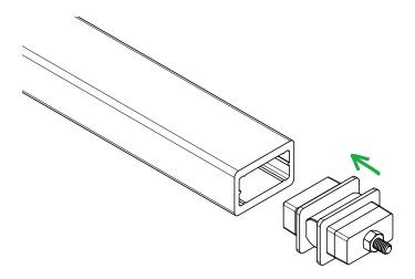
Set your Handrail Hinge straight (180°) and lock it in place by tightening the nut using a 7/16" socket or wrench. Slide part A into your handrail making sure the hinge pivots in the proper direction. The nut should be accessible. You may need to use a rubber mallet to gently tap the hinge into place.
