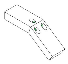
Finally, use a 1/8" bit (or appropriate) to drill 2-1/2" deep through the joint and into the opposite half of the spline.
