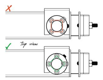
Insert the post top collar into the drill guide and use the set screw cutouts to position the holes in a **diamond** formation rather than a square so you don't interfere with your hinge plug.
