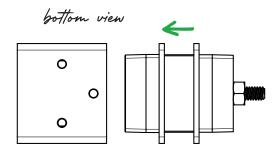
Set a Handrail Hinge straight (180°) and lock it in place by tightening the nut using a 7/16" socket or wrench.
