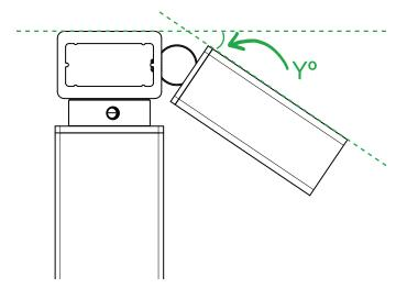
16 Set the Handrail Hinge to the pitch of your stairs (found in **step 3**). Carefully slip off the scrap handrail so you don't disrupt the angle of your hinge, and tighten the nut on the hinge using a 7/16" socket or wrench to lock the angle in place.
