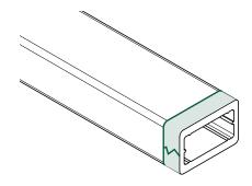
Apply painter's tape to your handrail to minimize chipping of the powder coat, and mark the cutting location and angle (if applicable).
