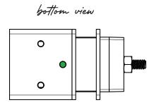
2 Secure the hinge by extending the pilot hole into the hinge plug using a 5/32" drill bit. Make sure to drill your pilot holes 1" deep into the handrail. Tap the pilot hole using the 10-24 tap.
