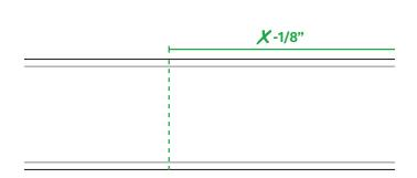
Using instructions for **Cutting Handrail** on **page 4,** make a straight cut at this location.
