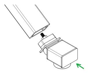
17 Slide one end of this piece of handrail over hinge part C of the stair end.
