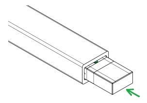
Slide a fixed straight spline into the end of your handrail that you need to continue until the dimple is flush with the end of the handrail. You may need to use a rubber mallet to gently tap the spline into place.
