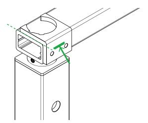
Pind the location of the Handrail Hinge by clamping the drill guide to the stair-facing side of your handrail with the edge flush with your straight cut and the post top template sitting on top of the handrail.
