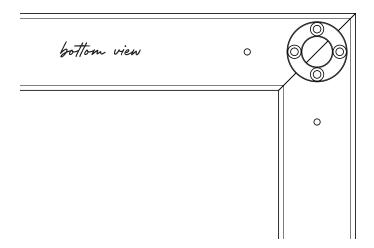
Remove your handrail and place it upside-down on your drilling surface. Attach the post top collar through the corner spline using the **End Post Tops** instructions on **page 25.** Make sure to drill your pilot holes deep enough into the spline to clear the 3/4" screws.
