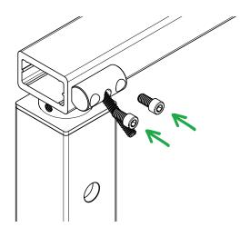
Align the flat side of hinge part B to the side of your post making sure the protruding screw pivots in the correct direction. Attach by driving in the two 1/4-20 x 1/2" socket head cap screws using a 3/16" Allen wrench.
