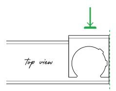
Find the location of your post top by aligning the edge of the Handrail Drill Guide and Template flush with the end of your piece of handrail and clamping it in place.
