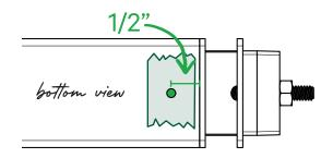
On the underside of the handrail, secure the hinge by drilling a 1" deep pilot hole 1/2" from the cut of the handrail using a 5/32" drill bit. Tap the pilot hole using the 10-24 tap. Drive in a 10-24 x 1/2" set screw by hand using a 3/32" Allen wrench.
