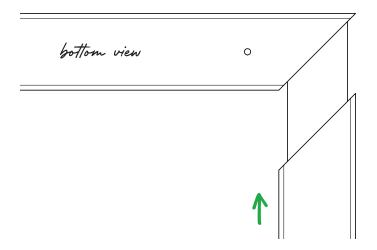
Flip the off-cut piece of handrail over and fit it to the installed spline to complete the corner.
