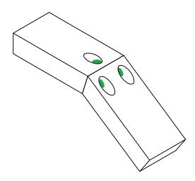
Check that nothing has shifted, and adjust as necessary. Switch to a 5/32" drill bit (or appropriate). Drill into each counter sunk pocket parallel with the opposite side and deep enough to accommodate the unthreaded shank of your screws.
