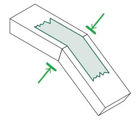
Flip over one of the halves and secure the two pieces together tightly using high-tack tape on the top and the bottom. Clamp the seam to keep the pieces from sliding side-to-side.
