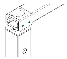
Drill the two pilot holes through the drill guide using a 7/32" drill bit. Tap both holes using a 1/4-20 tap.
