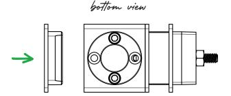
Slide an end cap into the other end of the stair end. It should fit snugly and does not need to be secured into place.
