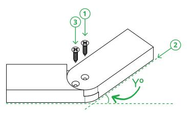
Assemble your adjustable horizontal corner spline using one of the included #8 x 3/4" pan head screws and a phillips head driver. Use an angle finder to set it to the angle of your corner transition (Y°), and lock it in place by driving the second #8 x 3/4" screw into one of the pre-drilled holes.
