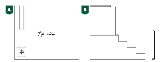
Certain sections may require multiple connections within a short span (under eight feet) and may need to be assembled as a unit before securing posts (C). This could be a short run with a corner or a stair transition. Assemble the whole unit and secure it to your posts all at one time. This will help you avoid removing anchoring screws in order to attach the end post tops.
