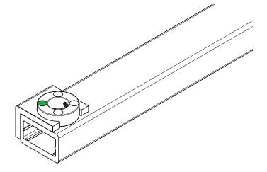
Mark the location of the first screw hole using a 11/64" drill bit then remove the post top collar.
