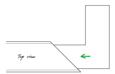
Slide a fixed corner spline into your mitered handrail. You may need to use a rubber mallet to gently tap the spline into place.
