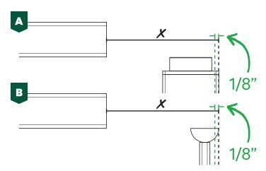
Working from the level section towards the stair transition, find the length of your handrail, and mark this length on a piece of handrail.
