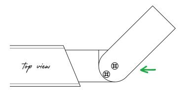
6 Slide the adjustable corner spline into your mitered handrail. You may need to use a rubber mallet to gently tap the spline into place.
