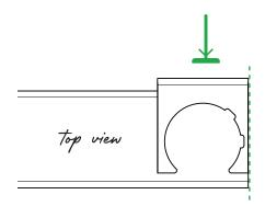
Find the location of your post top by aligning the edge of the Handrail Drill Guide and Template flush with the end of a piece of handrail and clamping it in place.
