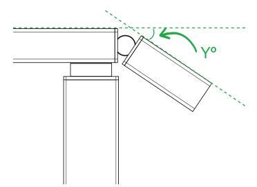
Set the Handrail Hinge to the pitch of your stairs (found in **step 3**). Carefully slip off the scrap handrail so you don't disrupt the angle of your hinge, and tighten the nut on the hinge using a 7/16" socket or wrench to lock the angle in place.
