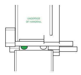
Using the 11/64" drill bit, drill the handrail through one of the post top holes. If your post top will be installed into an aluminum spline, drill 1" deep. If it will be installed into a delrin spline or without a spline, drill 1/2" deep. Tap the pilot hole using the 10-24 tap.
