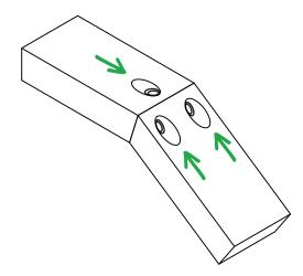
7 Drive in three 2-1/2" deck screws. Unclamp and remove the tape.
