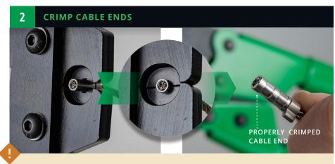
**CAUTION:** A properly crimped cable end is essential to maintaining the integrity and safety of your cable. A weak connection will slip over time or fail against an impact load!
