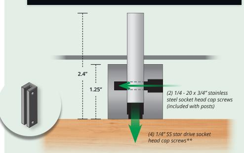
\*\*Post brackets MUST be anchored to project structural frame (joists, blocking, etc) and all 3" of Cable Bullet mounting screw threading should be engaged in structural material. If mounting directly to structural material, use 3-1/2" long mounting screws. If mounting through non-structural material (veneer or trim), use 4-1/2" long mounting screws.
