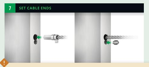
**CAUTION:** To minimize the risk of cross-threading or galling, use a manual socket screw driver or Allen wrench.
