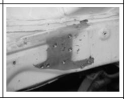
To properly attach the Hasport mount bracket on the frame rail, two holes will need to be drilled in the frame rail. Start by sliding the bracket over the frame rail so the holes at the bottom of the bracket line up with the torque mount holes on the bottom of the frame rail. Next mark the frame rail on the top using the mount bracket as a guide. After removing the bracket, use a 3/8ths inch drill bit and drill the two holes in the frame rail.
