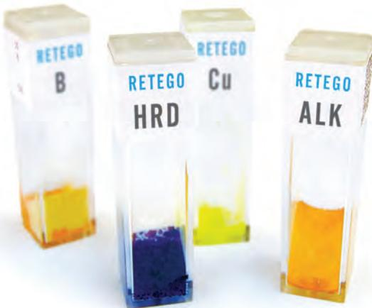
Single-use vials complete with stable chemical components. The only liquid involved is the 3ml water sample. Immediate digital results are ready for storage or distribution.
