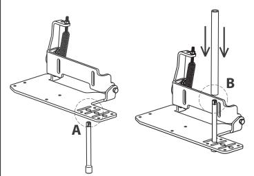
A) Slide a 3/8" drive extension into one of the holes in the hinge plate C) Step on the plate and pull the pipe toward you to bend the plate as needed. B) Use a piece of pipe over the extension for leverage
