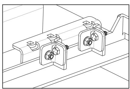
Tighten all bolts to secure platform to mower deck. You now have a secure platform to attach a low-profile GrassFlap to your Wright Aerocore mower.
