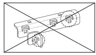
Loosely attach short angles to platform angle using 5/16"-18 X 1" carriage bolts. Leave 1/4" minimum gap between parts. Make sure cutout bolt holes are on top.
