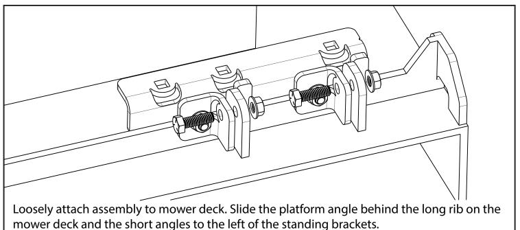
Tighten all bolts to secure platform to mower deck. You now have a secure platform to attach a low-profile GrassFlap to your Wright Aerocore mower.
