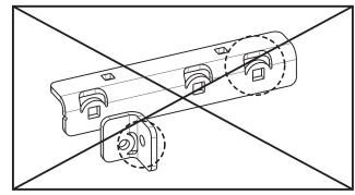
Loosely attach short angles to platform angle using 5/16"-18 X 1" carriage bolts. Leave 1/4" minimum gap between parts. Make sure cutout bolt holes are on top.
