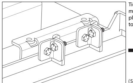
Tighten all bolts to secure platform to mower deck. You now have a secure platform to attach a low-profile GrassFlap to your Wright Aerocore mower.
