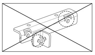
Loosely attach short angles to platform angle using 5/16"-18 X 1" bolts. Leave 1/4" minimum gap between parts. Make sure cutout bolt holes are on top.
