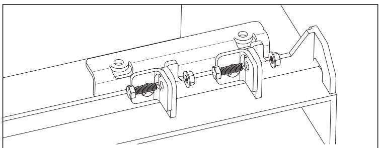
Loosely attach assembly to mower deck. Slide the platform angle behind the long rib on the mower deck and the short angles to the left of the standing brackets.
