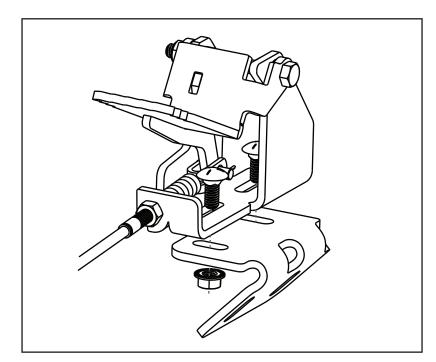
Mount pedal to pedal mounting plate 135 using 5/16-18 x 1 carriage bolts as shown.
