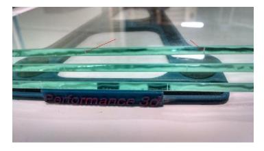
Slide the assembly under the rear clip of the build platform. Then carefully snap the front clips over the glass. Ensure all clips are over <u>top of the glass</u>. Make sure to <u>re-level the build platform</u> and enjoy printing on a totally flat surface!
