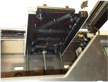
KEEP the **3 thumb nuts** and **springs**, you will re-use these! Remove the bag and masking tape from the underside of the new heated build plate. Also notice the 3 cutouts around the threaded posts, this is where the springs will sit.
