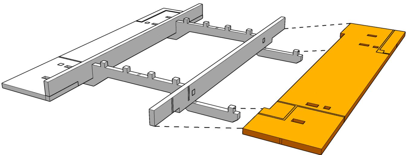
Align outer edges of the highlighted part then twist
