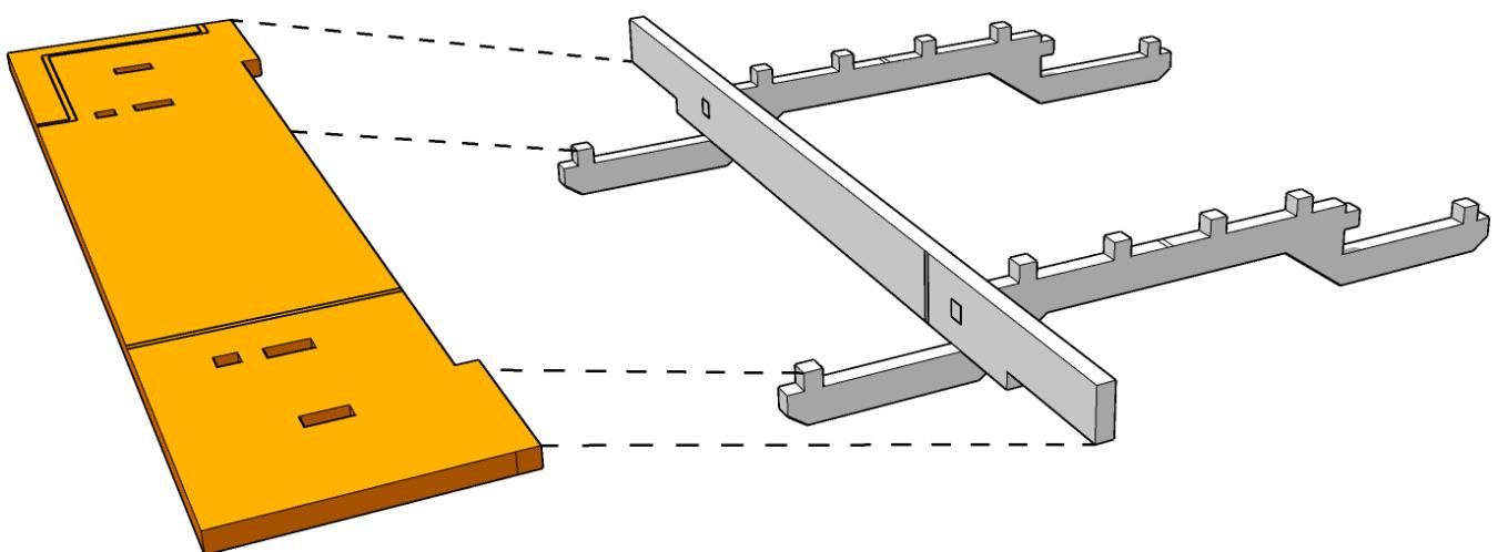
Align outer edges of the highlighted part then twist
