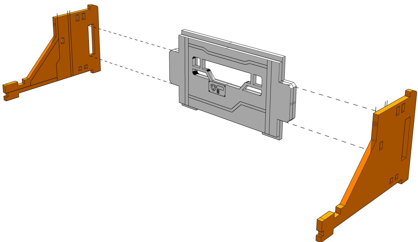
Detailing on both panels face inwards
