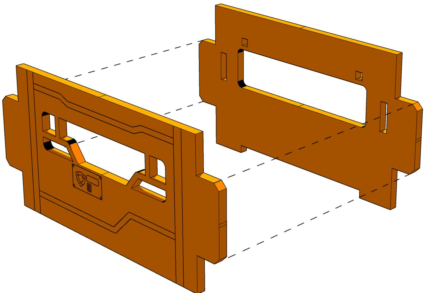
Detailing on both panels face outwards
