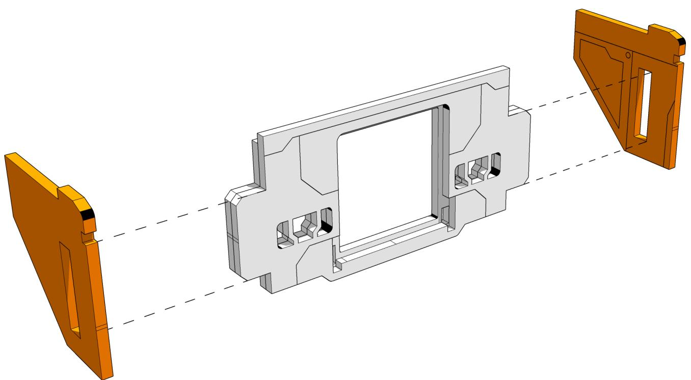
Highlighted parts are identical, detailing faces inwards
