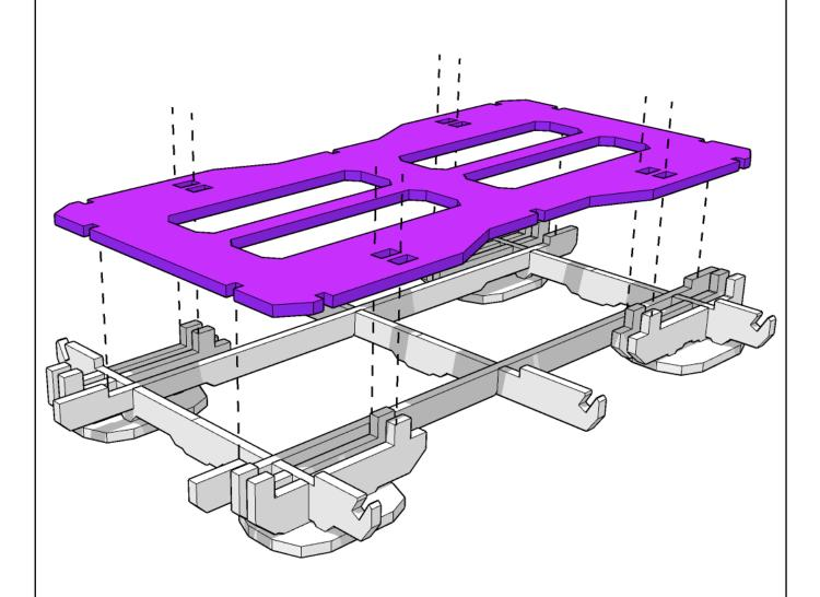
Feet will fit loosely within the tab holes. Glue to the long strips, not feet
