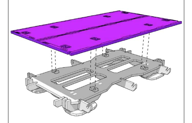
Recommended to glue the highlighted part to the support plate, not leg tabs. This allows for legs to be removable for the Skylevel leg kits.
