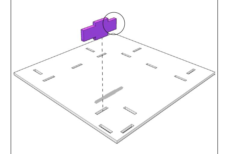
There are two similar parts. The circled section of the highlighted piece is shorter on one side and is the requited piece
