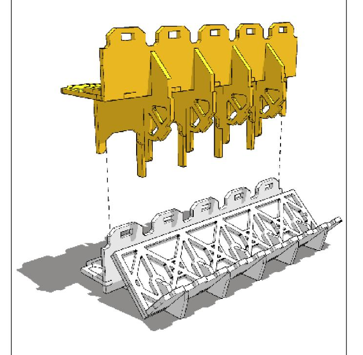
Upgrade slots over the straight. Gluing is optional.
