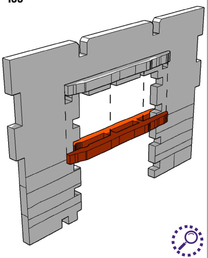
Highlighted parts shape matches the pieces above (fitted in previous steps). Make sure the circle cut out is in the same direction as shown above
