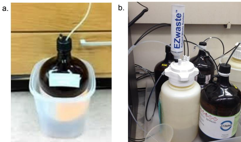
**Figure 2.** (a)<sup>10</sup> In order to prevent the waste container from building up pressure, a vent must be present in the system as shown on the left side of the cap. However, this makes the system open to release vapors into the air, contaminating the lab. (b) In order to trap the hazardous chemical vapors, an activated carbon filter can be attached to a specialized cap, as demonstrated. This will trap VOC emissions but allow filtered air to exit the container and relieve pressure.
