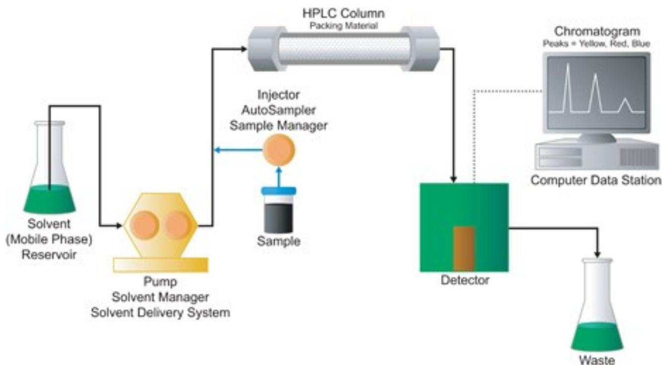
**Figure 1.** A diagram of how a HPLC machine functions.<sup>9</sup> Other variation of this simple method are used for different types of analyses. Solvent flows from a reservoir into a pump. It is then delivered to the column along with the sample where the two chemicals are separated based on affinity to the column. The detector determines the retention time for each chemical which can be used to identify the chemicals if necessary. The solvent is then deposited into a waste container.
