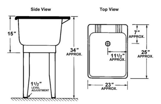
General: Furnish and install as shown on plans, UTILATUB® Laundry/Utility Tub model 14, as manufactured by E.L. Mustee & Sons, Inc. Tub shall be one-piece molded Co-PolyPure™ Tub complete with drain assembly and floor mounting hardware. White color, 16 lbs.
