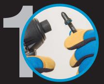
Choose bit size & attach it to the chuck or coupler. Fasten it well. Set power tool to MAX speed & torque if it is adjustable.
