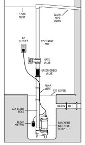
with the pit floor or wall. If the float switch does not move freely the pump will not activate.
