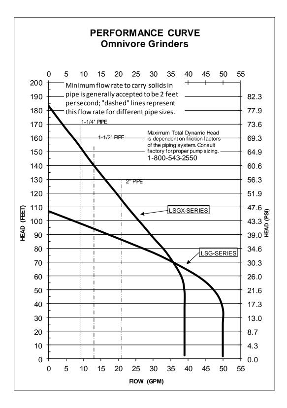
NOTE: Single stage units ("LSG" models) may not meet pressure requirements in all applications. Use of the 2-stage ("LSGX" models) may be required in certain applications. Consult factory for proper sizing and technical assistance where forced pressure mains or multiple homes tie into a common waste line.
