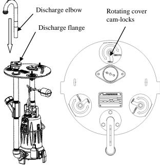
Although the Liberty Pumps RE/REX models come equipped with 6-pin connectors that mate perfectly with existing control hardware, the following table may be used for troubleshooting, repair, or custom installation purposes.
