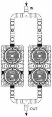
2 no. XL75 – PARALLEL Up to 150GPM, 1118 lbs Grease Capacity.
