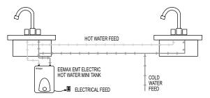
Point-of-Use Booster Heating Application from Central Tank Heating System
