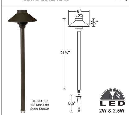
18" Aluminum pipe with 1/2" NPT on bottom. 12"
