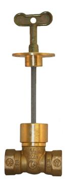
The C-67 AGA (American Gas Association) Gas Valve is for use on any gas fireplace or appliance. Using the included operating rod, the installer can install the valve from 1" to 14" depth, allowing it to be installed "below-the-joist," eliminating fittings and installation time. The C-67 Gas Valve is also used as a shutoff for any gas burning appliance.
