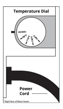
Manual Mode: Turn the dial in either direction to adjust your temperature up or down. Turn clockwise to increase temperature and turn counterclockwise to decrease temperature. Repeat this step until you achieve your desired temperature.
