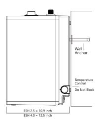
PLEASE NOTE: MINI TANKS ARE FOR INDOOR PERMANENT INSTALLATIONS ONLY, BEFORE POWERING THE WATER HEATER. BE SURE THAT THE SYSTEM IS COMPLETELY FILLED WITH WATER AND ALL AIR IS REMOVED. THIS MANUAL AND ALL ECCOTEMP CONTENT IS SUBJECT TO CHANGE WITHOUT NOTICE. PLEASE VISIT SUPPORT ECCOTEMP COM FOR MORE INFORMATION.
