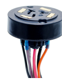
K171H Locking Type Receptacle, 7-Pin, C136.41 Compliant, 12" lead
