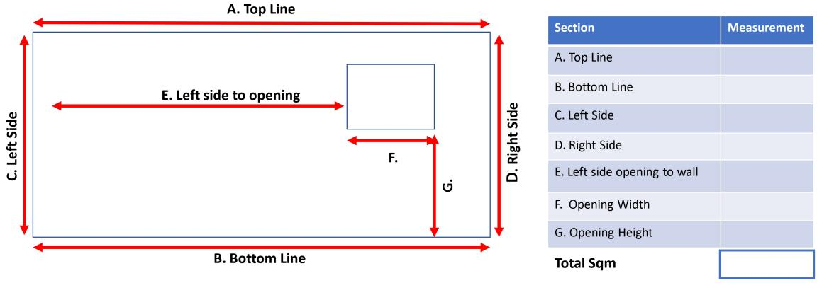
Measure each length as indicated by each red arrow, tip to tip. We can determine the cut away with these measurements.
