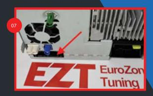
08-Connect the camera's power wire to your 10amp mini add-a-fuse (pictured). Locate an applicable fuse (Fuse 24 used in this example)
