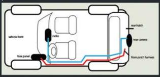
06- Remove the RCD510, RNS510 or RNS315 to gain access to the rear of the unit. This is where you will install the 26-pin harness.
