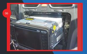
07- Route the 26-pin connection to the rear of the RNS510, RCD510 (H or F), or RNS315. Reinstall the Radio back into its stock location.
