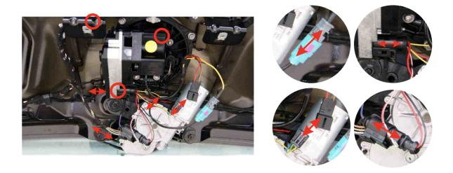
Utilize this guide to help with tapping into the taillight for trigger (yellow wire in our kit) as well as feeding the cables through to the interior and to the back of the radio.
