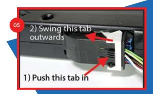
05- Remove the harness from your existing Bluetooth module by pressing the tab shown and swinging the white connector outwards.
