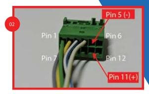
03) Flip the tab on the side of the green block to access the pins. You can now insert a wire into the green harness. Reinstall is the reverse of removal.
