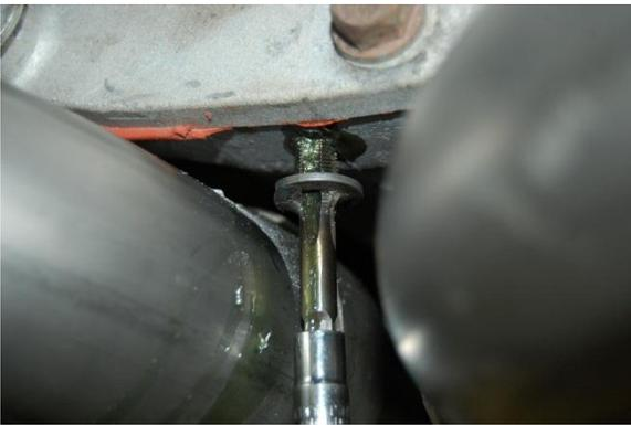
7. Start the 1/8" NPT tap into the hole at the approximate angle that the drill bit went into the differential housing- to the stop on the tap. The hole needs to be at an angle of at least 15° to miss the bottom differential cover bolt; it also aids drain plug access.
