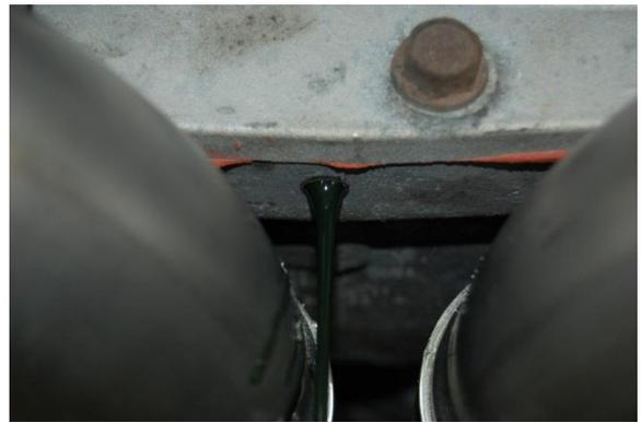
6. When the fluid stops draining, finish drilling until you reach the stop point on the drill bit.
