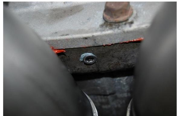
10. Fill the differential with Mobil 1 75W90 synthetic or your choice of fluid. A bottle of GM limited slip additive is also recommended.
