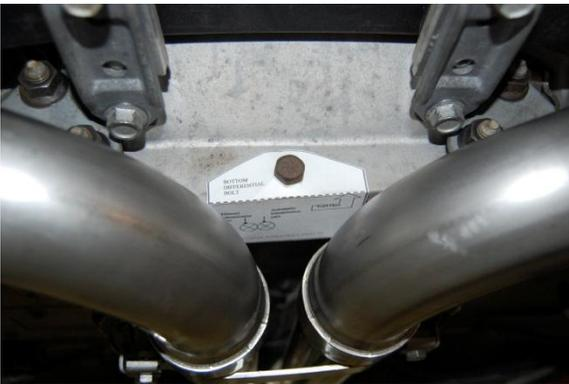
3. Place the template over the bottom differential bolt.
