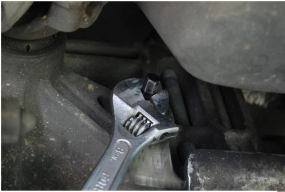
1. Remove the differential fill plug.
