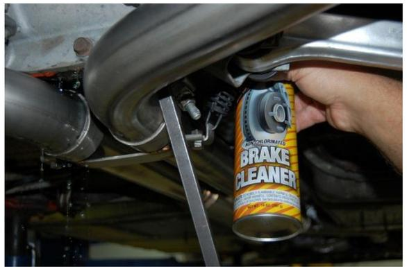
8. Flush the differential with brake cleaner at least twice. Use the brake cleaner to clean the outside of the differential and the exhaust pipes as necessary.
