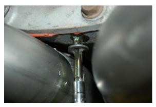
7. Start the 1/8" NPT tap into the hole at the approximate angle that the drill bit went into the differential housing- to the stop on the tap. The hole needs to be at an angle of at least 15° to miss the bottom differential cover bolt; it also aids drain plug access.
