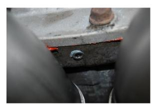
10. Fill the differential with Mobil 1 75W90 synthetic or your choice of fluid. A bottle of GM limited slip additive is also recommended.
