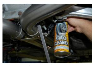
8. Flush the differential with brake cleaner at least twice. Use the brake cleaner to clean the outside of the differential and the exhaust pipes as necessary.
