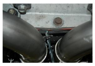
5. Start the 5/16" drill bit; drill in approximately 1/8." Once the drill bit starts, angle the bit 15° towards the center of the Y-pipe. Drill in 1/2" until the fluid starts to drain.
