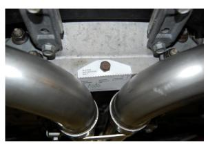
3. Place the template over the bottom differential bolt.
