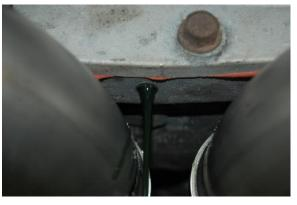
6. When the fluid stops draining, finish drilling until you reach the stop point on the drill bit.
