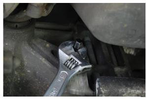
1. Remove the differential fill plug.
