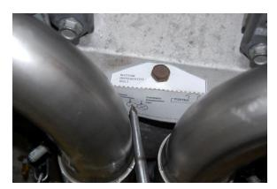
4. Center the punch on the template. 15mm hexhead manual transmission cars use outboard hole; 13mm hexhead automatic transmission cars use inboard hole.
